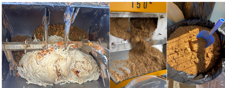
Figure 5. Final dry animal food product obtained from Type B processing in the ECOAIR 150 device.
