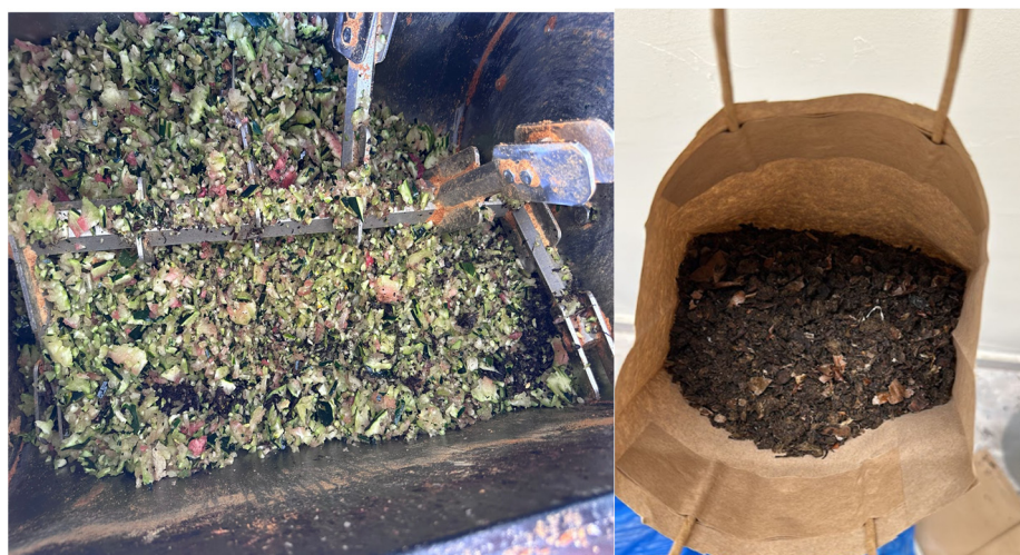
Figure 4. Shredded organic waste inside the ECOAIR 150 during Type A compost processing.
