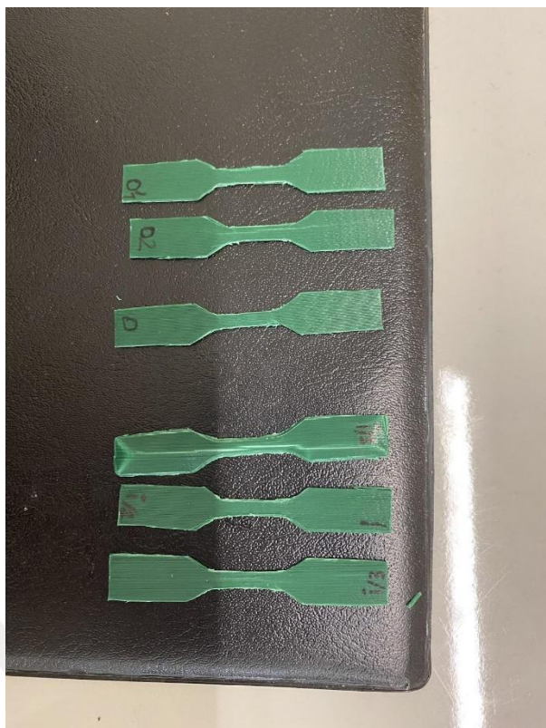
Figure 3.9 Dumbbell shaped 3D printed food pack wall samples
