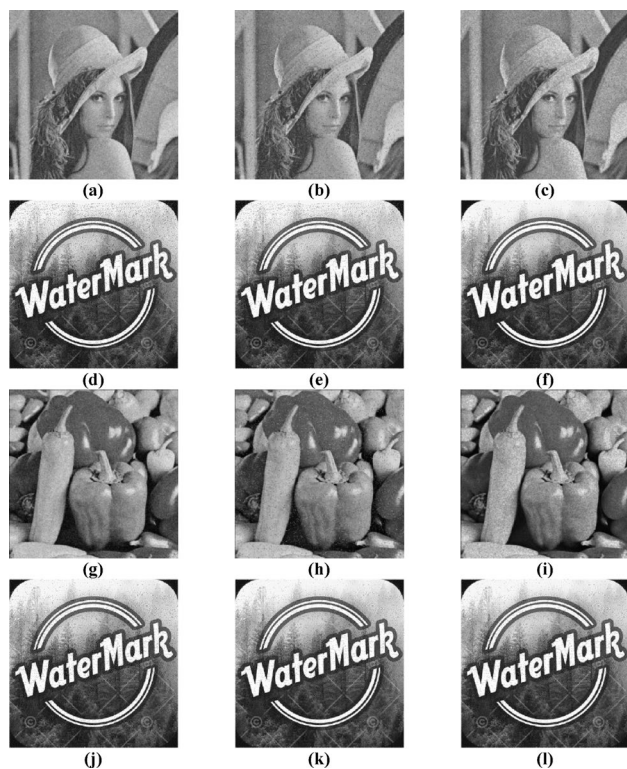
Fig. 8 Sample attacked watermarked images and extracted watermark: (a)–(c) noisy watermarked Lena with Gauss (0.01), Salt & Pepper (0.05) and Speckle (0.05), respectively, (d)–(f) extracted watermark from noisy watermarked Lena, (g)–(i) noisy watermarked Peppers with Gauss (0.01), Salt & Pepper (0.05) and Speckle (0.05), respectively, (j)–(l) extracted watermark from noisy watermarked Peppers
