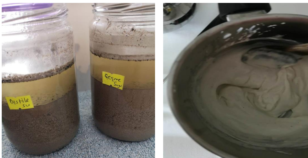
Figure 1: The ash water (a), saponification of oil with ash water (b).
