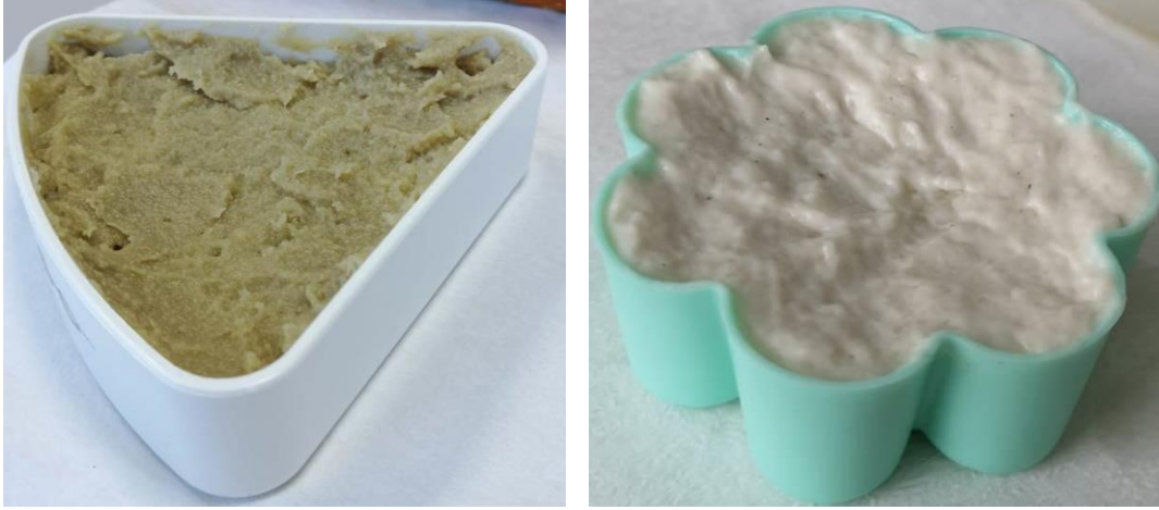
Figure 2. Pouring the soap paste into molds and leaving it to dry.
