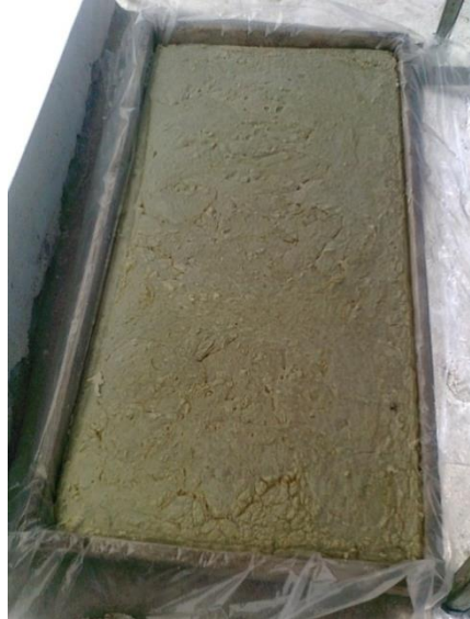
Figure 3. Drying of soap in molds with fixed height and nylon coated [14].
