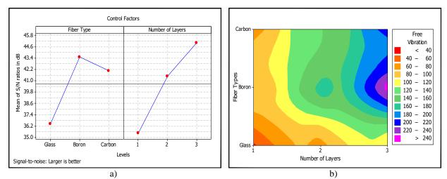
Figure 3. a) effects of control factors for S/N ratio data and b) contour plot of fundamental natural frequency
