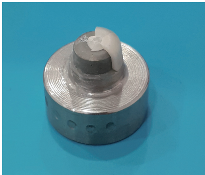
Fig. 2 Fracture pattern of zirconia restorations
